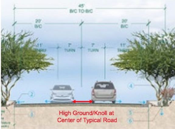
FIGURE 26: TYPICAL STREET CROSS SECTION
